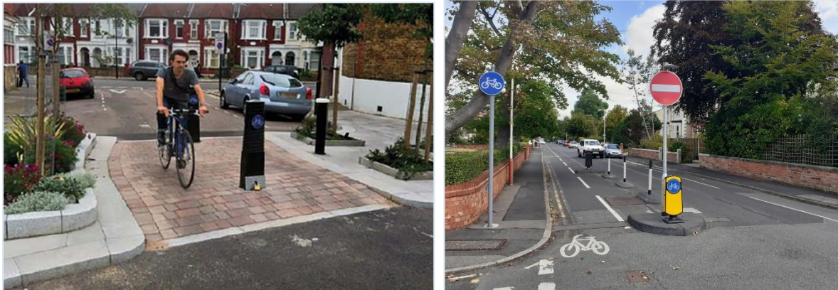
Figure 6-14 - Temporary (Left) and Permanent (Right) Modal Filter
