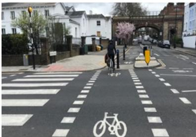
We want to make it easier for walkers and cyclists to cross the road so we will put a Tiger crossing. A Tiger Crossing works like a Zebra Crossing but with an extra space for cyclists. Traffic must stop for walkers and cyclists to cross. This will be across Scarisbrick New Road at the junction with Hampton linking to the cycle lanes and footways on either side of the road.
