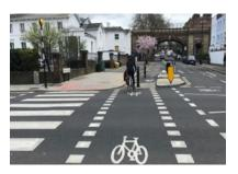
We want to make it easier for walkers and cyclists to cross the road so we will put a Tiger crossing. A Tiger Crossing works like a Zebra Crossing but with an extra space for cyclists. Traffic must stop for walkers and cyclists to cross. This will be across Scarisbrick New Road at the junction with Hampton linking to the cycle lanes and footways on either side of the road.
