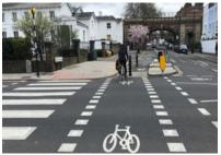
We also want to make it easier for walkers and cyclists to cross the roads so we will ban cars from turning left from Norwood Road into Tithebarn Road to allow a crossing point for walkers and cyclists, making it safer to cross the road. We will also put an advanced cycle stop line - this is a space in front of the traffic and set of traffic lights that allow cyclists to go before cars, vans and lorries. This will be on Bispham Road and Tithebarn Road
